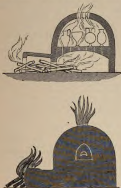
FIG. 9.—Potter's kiln; elevation and conjectural section. Early Greek: the Egyptian kiln is narrower and taller, and has no dome.
